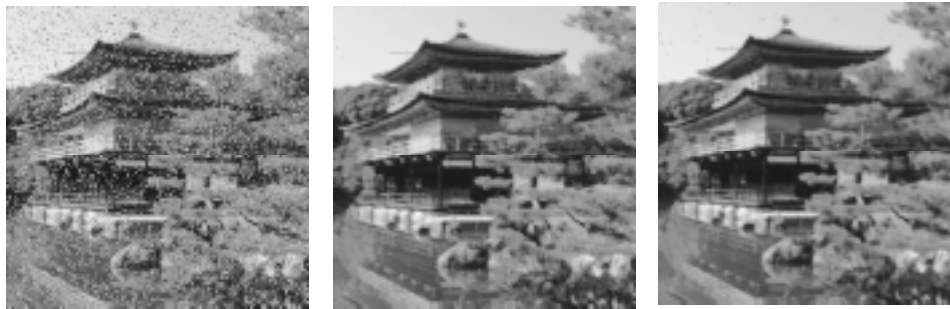
Figure 1. Impulsive noise filtering using a preliminary exponential noise detector. (a) The input image is corrupted by impulsive noise (15% corruption rate); (b) the result of filtering using the exponential noise detector; (c) the result of filtering using the simple median filter.
